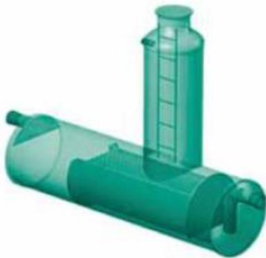
An oil-and-petrol separator is intended for trapping and accumulating petroleum products and suspended from surface waster waters.
