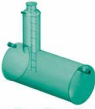
A sand separator is a cylinder-shaped vessel with connection pipes for intaking and discharging waste waters. A level-monitoring device may be inbuilt to check accumulation of sand. Maintenance of the sand separator is carried out through a service manhole.
