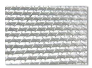
ARMATON multiaxial fabric is a textile material consisting of one or more layers of glass fibers. The layers are oriented in various directions and stitched with a polyester yarn. ARMATON multiaxial fabrics are manufactured using state-of-the-art equipment from Germany, which quarantees output of high-quality products.
