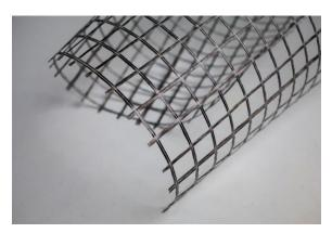
**BENSTEN K basalt masonry grid** is a flat rolled reticulate material comprising elastic ribs of hightensile basalt yarns bound together with a knitting yarn at the nodes to form rectangular mesh. The grid is impregnated with special agents to improve its properties and enhance its stability. Mesh size depends on intended purpose of a grid.
