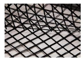
**HIGHWAY geogrids** are two systems of yarns interknit with a third one (knitting yarn). Geogrids are impregnated with polymer dispersions and may be made of glass, polyester or basalt yarns
