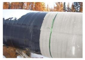
*GRINCODE* multiaxial rockshield is a composite manufactured using up-to-date high-strength glass-fiber and synthetic nonwoven material and impregnated with environmental friendly thermoplastic resins.
