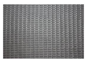
**Woven geotextile «GRUNTSTAB»** – is a material made by textile technology (weaving and knitting) of high modulus polyester yarns.
