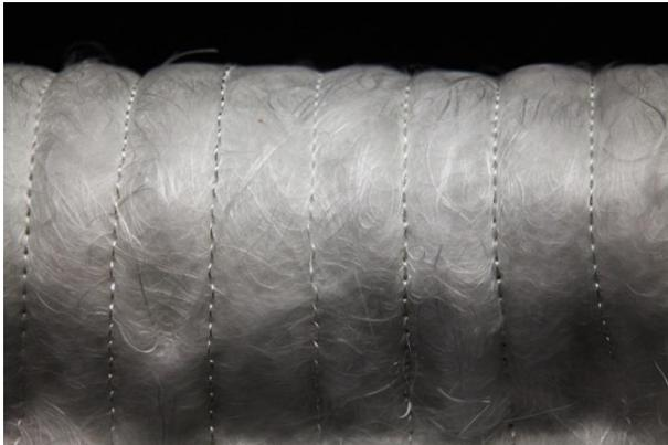
**PSH-T stitch-bonded glass-fiber nonwoven fabric** is a multi-layer web stitch-bonded by franse or tricot weave. PSH-T stitch-bonded nonwovens are intended for thermal insulation.
