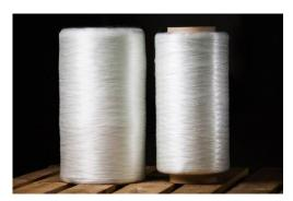
**Voluminized roving** is a roving drawn through an airjet nozzle that imparts continuous bulk.
